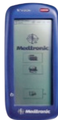
Fig. 13: Programmer for postoperative programming of pacemaker (pulse generator)
